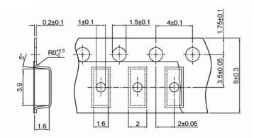
Accumulated pitch tolerance is ± 0.2 mm over 10 pitches
