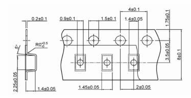
Accumulated pitch tolerance is ± 0.2 mm over 10 pitches
